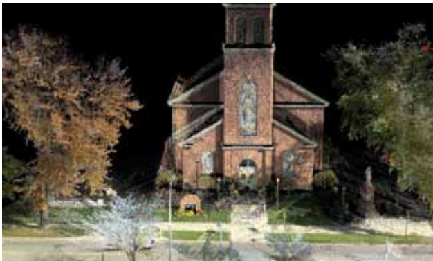
Mobile LiDAR combined with street-level photography used to create the City of Monroe's tree inventory. (Photo credit: City of Monroe, Michigan)
